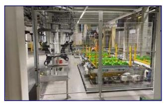
The axle carriers are transported through the system with the help of a Power & Free system consisting of 5 chain circles. At the loading station, the axle carriers are removed from transport boxes with the help of handling robots and transferred to the P&F system. The axle supports are transported into the painting booth through a masking area. After painting has been completed, the transport route leads through an evaporation zone into the dryer. Here the painted axle carriers are dried at a
