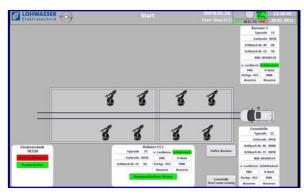
The bodies painted with the base color are prepared for the second painting in a masking station. In this station area that are not to be painted again were masked with paper or foil. After this work step, the target "2-tone painting" is written on the data carrier of the body. The destination control now drives the body back into the paint shop with the help of the conveyor system. At the entrance to the
